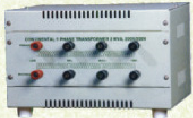
1 ph Air cooled Transformer
